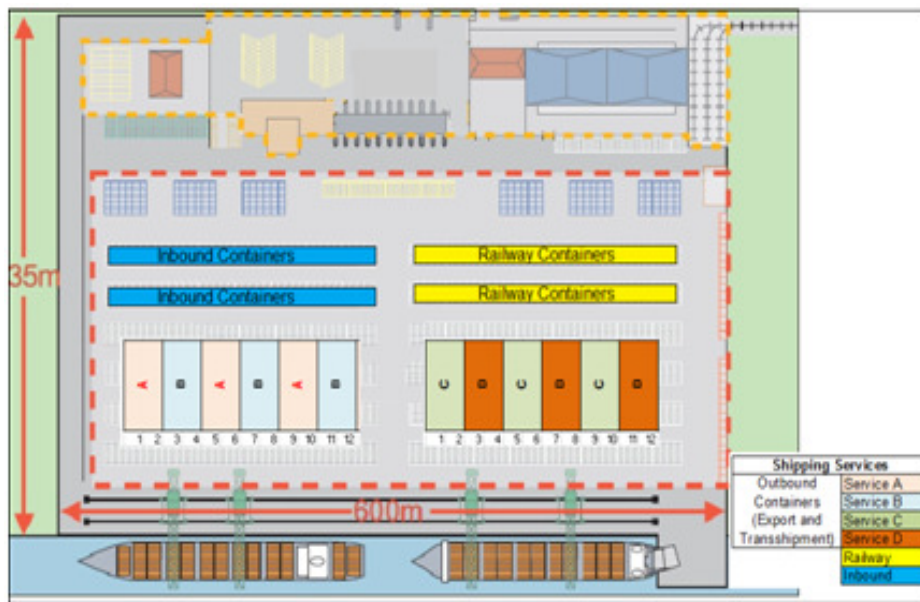
Figure 3: Storage Yard Layout for a transshipment container terminal. Higher detail in stacking criteria and configuration of storage blocks [8]
